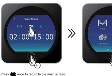
$\wedge$ NOTE: The setting step is "hour to hour". Once the Timer is activated, it is active for all seven days of the week.
